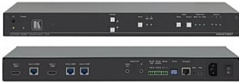
The VM-212DT is 4K@60Hz (4:2:0) HDMI & extended-reach HDBaseT DA for HDMI and HDBaseT signals. It reclocks and equalizes the signal and distributes it to two identical HDBaseT outputs and a looping HDMI output. It supports resolutions up to 4K@60Hz (4:2:0). This product offers the versatility of control options and audio de-embedding
